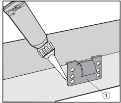
■ Coat the side and lower edges of the spring clips between ① and ② with silicone.
